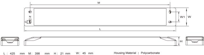
$W1: \ 22 \qquad mm \quad N : \ 4.2 \qquad mm \quad Q : \ 7.2 \ mm \\ Slot \ On \ One \ Side \ Allowing \ Alignment : \ M+/-3 \ mm \\ Tolerance : \ +/-1 \ mm \\$
